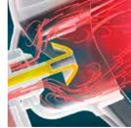
Cork-Shaped Pin Directing the Oxygen Flow
