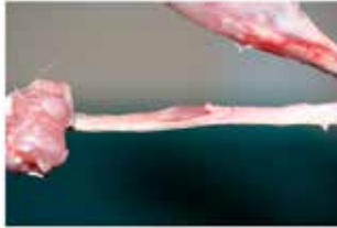
Figure 2: Tendon stretching with tensile force application in the apparatus
