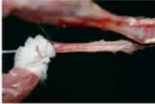
Figure 1: Start of the application of tensile forces to the Achilles tendon in the apparatus
